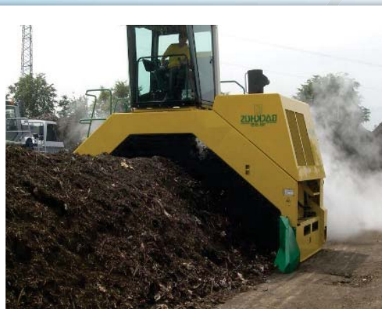
Machine for compost mixing
